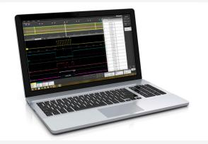
TekScope emulates the operation of a 4, 5 or 6 Series on your PC. The starter license enables you to view and analyze waveforms, make measurements, remotely access your oscilloscope, and decode I<sup>2</sup>C, SPI and RS-232.
