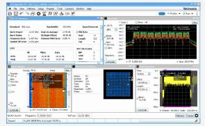
SignalVu-PC turns your Windows-equipped 5 or 6 Series MSO into a wideband vector signal analyzer. It can be customized to suit your appplication.
