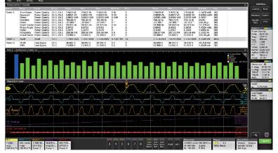
Power analysis packages enable automatic measurement of harmonics, switching loss and other key parameters.
